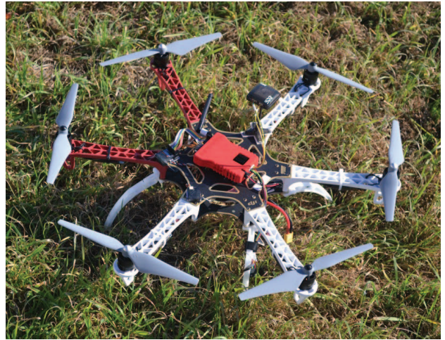
Fig. 7: IntelinAir RD-100 Hexacopter
